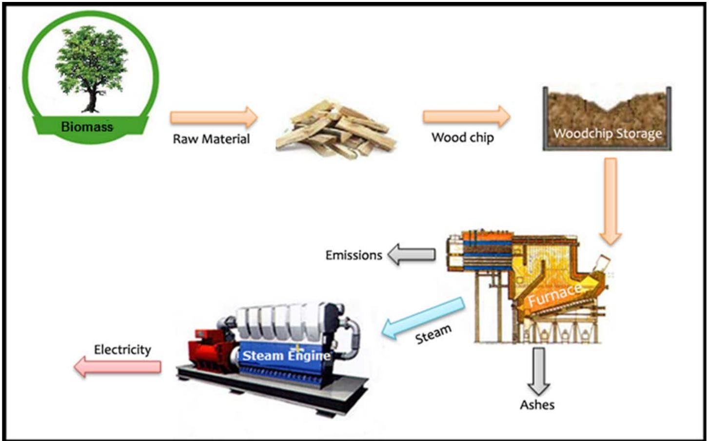
**VAP System** has insignificant air pollution, that comes from woodchips combustion in the furnace. The system is equipped also with a cyclone filter to complete emission abatement.
